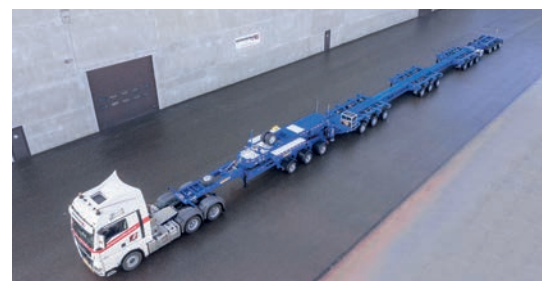
The HighwayMax Dolly&Booster is composed of nine hydraulically steered pendular axles, a 3-axle jeep dolly and a 3-axle nitro booster
