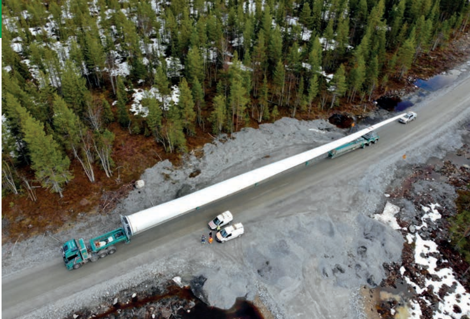
Uddevalla Specialtransporter using its Faymonville WingMAX in Piteå, Sweden to move a 69 metre blade
